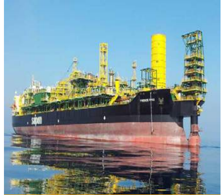
FPSO (Floating Production Storage and Offloading)
